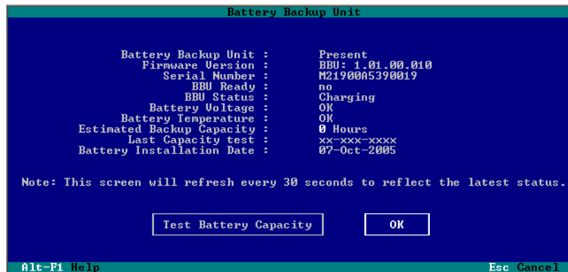
Figure 88. Battery Backup Information Screen in 3BM
