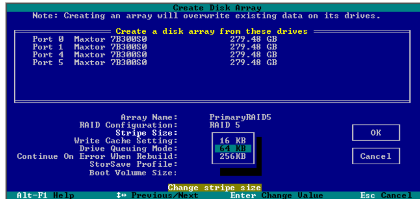
Figure 14. Stripe Sizes for a RAID 5
